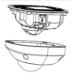
Figure 2-17 Remove the Front Cover
