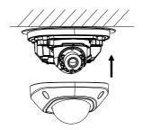
Figure 2-6 Install the Front Cover
