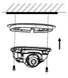
Figure 2-4 Fix the Camera Body
