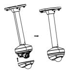
Figure 2-12 Install the Front Cover
