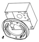
Figure 2-7 Fix the Adapter Plate
